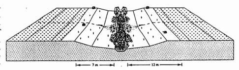
The natural physical dimensions of riffle pool associations should be set so to have one pair, a riffle and a pool, at a downstream distance of 5-7 times the stream width.
