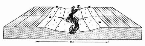
A meandering channel by definition is one that has a channel length that is at least 1.5 times the length of the down valley distance. Since many stream processes can be quantified on a length basis, the longer channel has greater purification properties.
