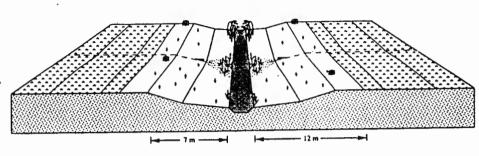
simple recommendation to limit this, is to reduce the stream channel side slope from the present 50% (i.e. 1:2) slope to a minimum of 25% (1:4) slope as shown in the figure.
