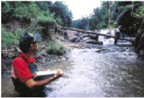
Figure 8.49: Surveying a stream. Channel surveys establish baseline information needed for restoration design.
