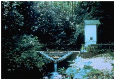
Figure 7.9: Station measuring discharge. Permanent stations provide measurements for a wide range of flow, but the necessary measurements can be made in other ways. Source: C. Zabawa.
